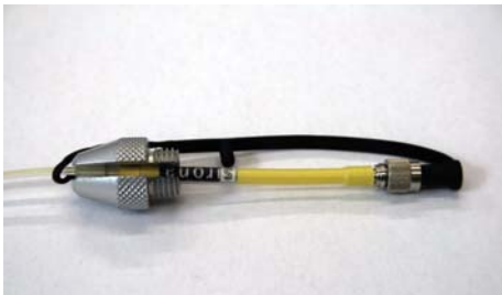
Figure 13: Optical fiber with protection caps
