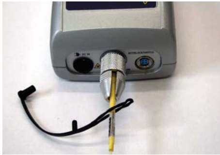
Figure 15: Connecting the optical fiber
