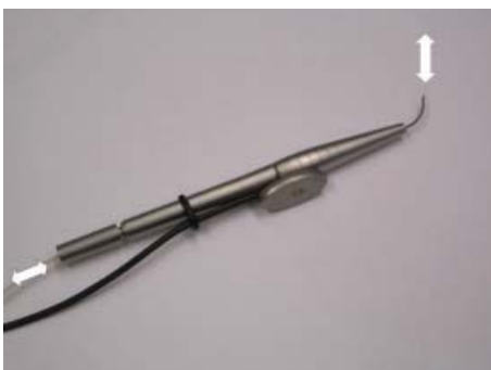
Figure 19: Adjusting the length of the optical fiber
