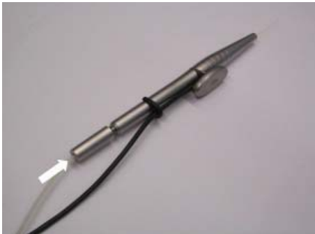
Figure 17: Inserting the optical fiber into the handpiece
